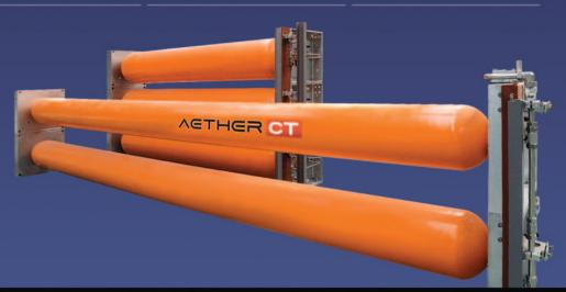
H2 storage vessels are offered with high pressure (FP 400~500 bar) and ultra-high pressure (FP 875 bar) products to hydrogen filling stations and can be manufactured as two-stage or three-stage cascades.
