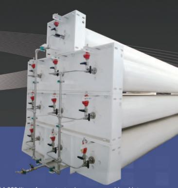
These storage vessels are mainly used for H2 and CNG, industrial factories and ships. Usually three vessels of 1,300 liters for content volume are combined into one module. In the case of large storage stations, several modules can be installed together. The specifications for vessel design, manufacture and inspection comply with the ASME standard of the USA, as well as the standard of the Korea Gas Safety Corporation. These vessels are manufactured and exported to countries all over the world.
