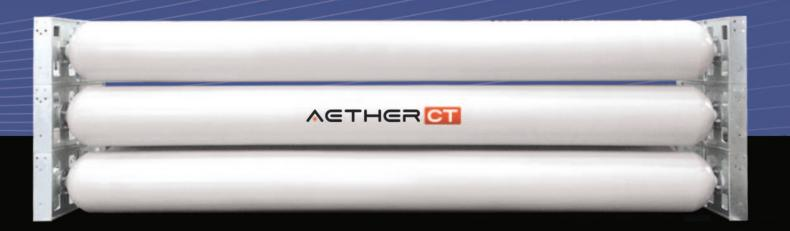
AETHER CT has delivered various Air Pressure Vessels to customers in order to obtain constant tension in the marine drilling riser. Air Pressure Vessel is connected to the Piston accumulators air-side in Marine riser tensioner system. This means that the riser tensioner unit acts like a hydro/pneumatic spring by using the compressed air from Air Pressure Vessel. These ultra high pressure vessels have also special demands from aerospace centers for rocket launching program.
