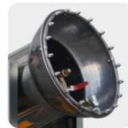
18 nozzles help to spray out the liquid widely
